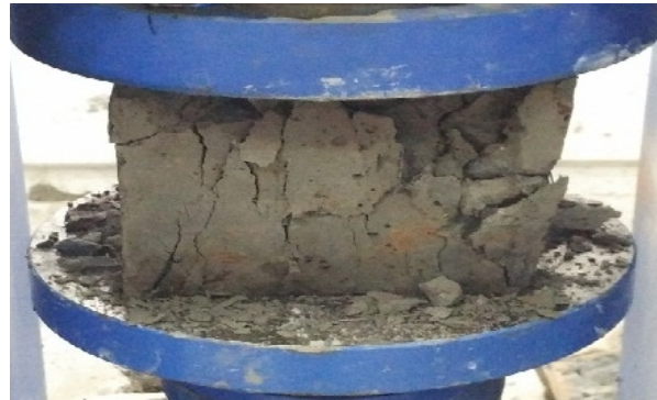
Fig. 1. Cube Under Compression Testing Machine (Ctm).
